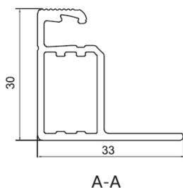
SOPRASOLAR FIX EVO – TAN DTU, SOPRASOLAR FIX EVO TILT – TAN DTU
